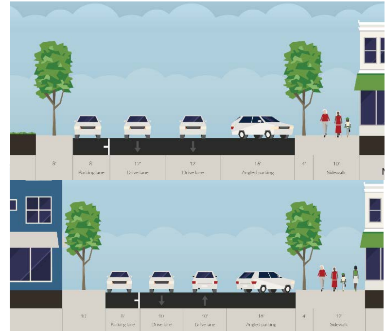
Figure 7 Clark St looking east between Sherman and Orrington. Top: current (1-way) configuration with Oldberg Park. Bottom: Future configuration (2-way) with new Civic Center building
